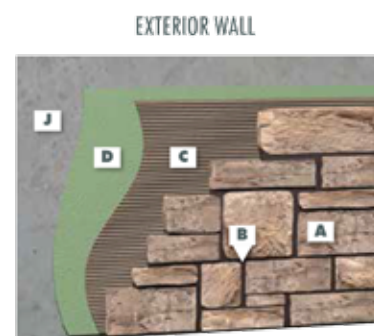
Concrete wall — Direct adhered with fluid applied MVIS™ Air & Water Barrier
