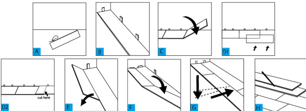
Always check flooring planks for defects such as chips and color variations under good light conditions. Check that grooves are free of debris. **Use planks from multiple boxes** during installation to insure random pattern variation.
