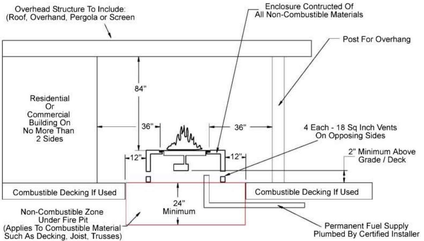
**Diagram Below Used For Fire Pits Ranging From 201,000 BTU Up To 400,000 BTU**
